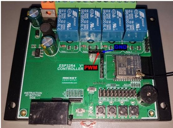
Use an SSR which can be controlled by a 3.3V PWM signal, and use a controlled device that is suitable for variable control via the used SSR.
